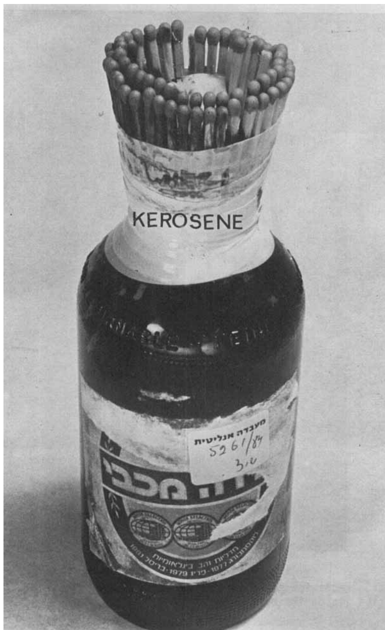
FIGURE 3 A "crown of matches" - type ignition mechanism.
